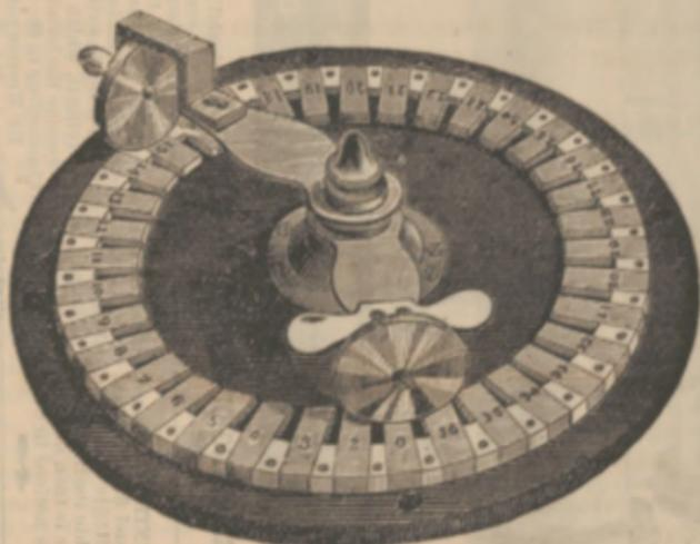
Enlarged view of the great circle, wheel-armed compound switch, selector of consecutive numbers of batteries, and to increase or diminish the number of cells included, either with or without interrupting the circuit. This differs from all other current switch cell selectors, in its adaptation to throw out of the circuit, any number at the beginning, as well as at the end, of the series. Patented.
