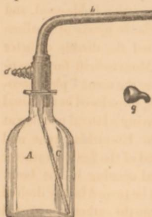
ment is of hard rubber and consists of a tube *b*, enclosing a smaller tube which communicates with the dip-pipe *c*. At *d*, a flexible tube with double bulbs is connected, by which air is forced into the atomizer. At *e*, mouthpieces of different shapes can be attached by screwing them on to the tube, and by varying the position of the openings in the mouthpieces the jet
