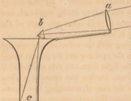
The advantage of the prism over a mirror or other reflecting surface is, that we have almost total reflection, and but little of the light concentrated upon the prism by the lens is lost.
