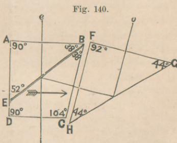
square, and the side of the square which is equal to DC, should be six-tenths of an inch. The remaining dimensions will be determined by this, and by ED, which should be three-twentieths of an inch. The surfaces of section, BE, may be brought very near to each other. In the construction actually employed they have been separated only by a single thickness of tinfoil, introduced at each of the angles.
