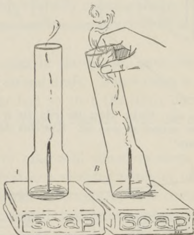
FIG. 104. Why does lifting the chimney make the joss stick burn better? Would a fire burn well in a wigwam if the wigwam could be tightly closed at the bottom?
