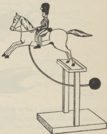
FIG. 41. The ball of lead in this toy balances the horse and rider because the weight is the same.
