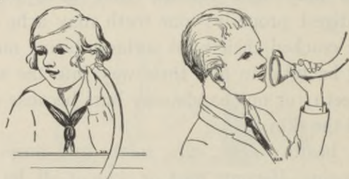
FIG. 142. When the boy talks into this speaking tube made with two funnels and a long piece of hose, the sound waves travel to the other funnel and reach the ear of the girl who is in another room. When the girl's eardrum catches these waves she hears what the boy is saying.
