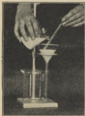
FIG. 13. Pouring into a filter.
