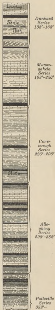
FIG. 74. Section of the coal measures in Ohio. The black bands represent coal beds. (U. S. Geol. Survey.)
