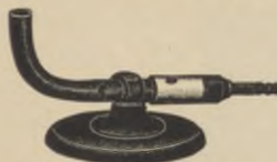
FIG. 2. Bunsen burner, low form.
