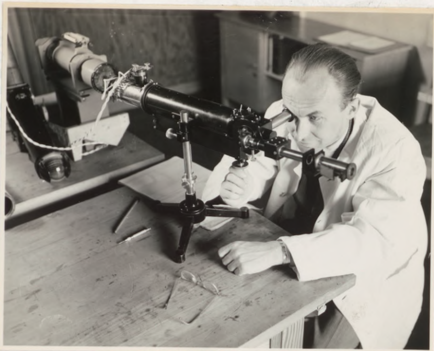
The possibility that all individuals are myopic under conditions of very low illumination was studied by Dr. Heinrich Rose, former Luftwaffe flight surgeon, who has worked extensively on night vision. He is shown above making an adjustment in the newly developed Engelking-Hartung adaptometer using the Schmidt-Haenesch photometer. The relationship between blood dynamics in arteriovenous fistulae and collapse under high accelerative forces led Dr. Otto Gauer, center, below, to study a group of patients with arteriovenous fistulae. He is shown here recording blood pressure and speed of pulse wave in patient, left.
