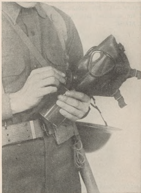
FIGURE 74.—TWO. Examining outlet valve.
