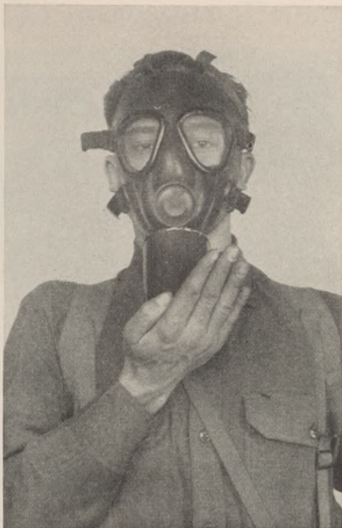
FIGURE 67.—CHECK MASK. Stopping inlet valve.
