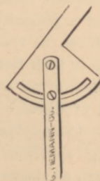
FIG. 5.—Stillman's joint movement for fixation or motion.
