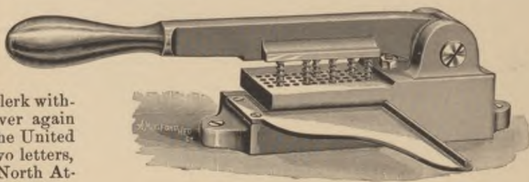
FIG. 3.—THE HOLLERITH GANG PUNCH.
